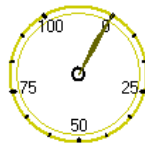
Figure 4-47 Circle Meter (TP70 series text panel)
